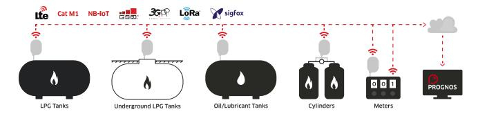
ISA is an **IoT company for Oil&Gas** specialised in remote monitoring solutions. Our solutions are based on data loggers that collect data and send it to ISA IoT Platform - Prognos - through **2G**, **3G**, **LTE-M**, **NB-IoT**, **SIGFOX or LoRa** networks.
